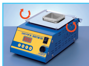
Loosen the screw on both sides.
