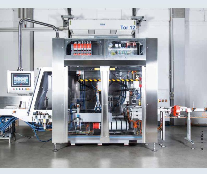
Cartoning machine with conveyor technology
