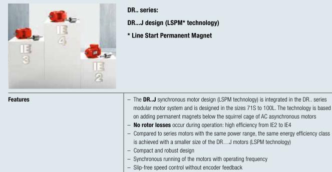
DR.. J LSPM motors can be operated with the frequency inverters MOVITRAC<sup>®</sup> LTE-B and MOVITRAC<sup>®</sup> LTP-B, MOVITRAC<sup>®</sup> B, MOVIFIT<sup>®</sup> FC and MOVIMOT<sup>®</sup> D
