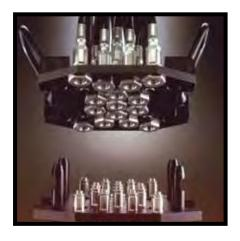
Typical hydraulic control curcuit panel incorporating twelve 3/8" BN semi balanced couplings and three 1/2" BN semi balanced couplings (no additional separation force when pressurized). Two plate system utilizing cam-locking devices.
