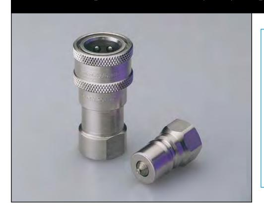
Snap-tite's 72 Series may be used in a break-away harness for compressed natural gas (CNG) fueling systems due to the "superior poppet sealing" designed specifically for compressed natural gas. These couplings feature superior pressure and flow characteristics over other manufacturers while meeting or exceeding the ISO-7241-1 Series B specifications.
