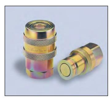
The 71 Series couplings are designed for today's applications including special features for modern needs - dry break, push-to-connect, high pressure, rugged & versatile. Extra large flow chambers and Snap-tite's exclusive valve design permit exceptional flow while maintaining low pressure drop.
